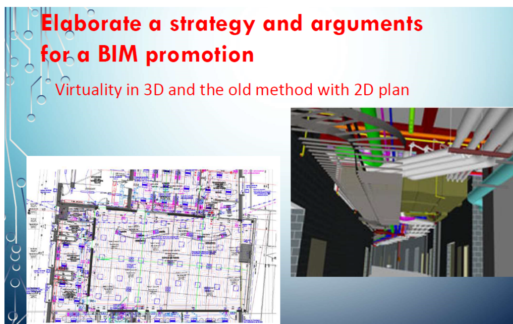
Illustration 1 : comparison between a complex 2D plan (left) and a 3D-vision (right)
