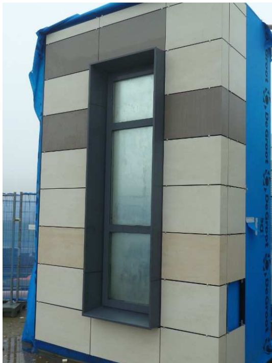
Mockup façade for airtightness test
